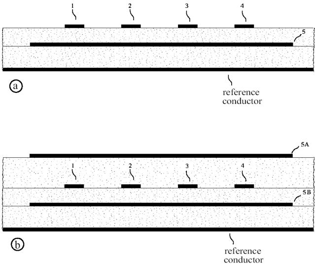
Fig. 4. Two possible cross-sections for the interconnection used in the ZXnoise method, where 1 to 4 are the TCs, where 5 is the RC in the coplanar-strips-over-return-conductor structure (a) and where the RC is made of the conductors 5A and 5B in the coplanar-strips-inside-return-conductor structure (b).
