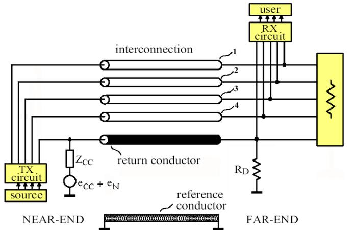
Fig. 2. A PDL with voltage-driven common conductor. The block containing the resistor symbol is a termination circuit.
