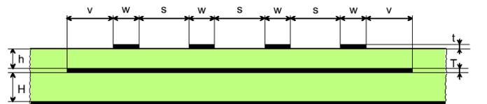
Fig. 3. Cross-section of an interconnection-ground structure built in a printed circuit board.
