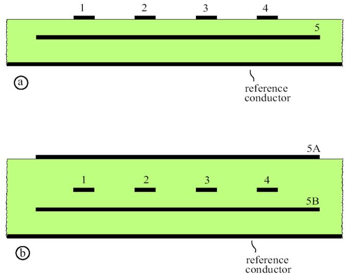
(1) Fig. 1. Two possible cross-sections for an interconnection-ground structure used with floating termination circuits, where 1 to 4 are the TCs, where 5 is the return conductor in a and where the return conductor in b is made of 5A and 5B.
