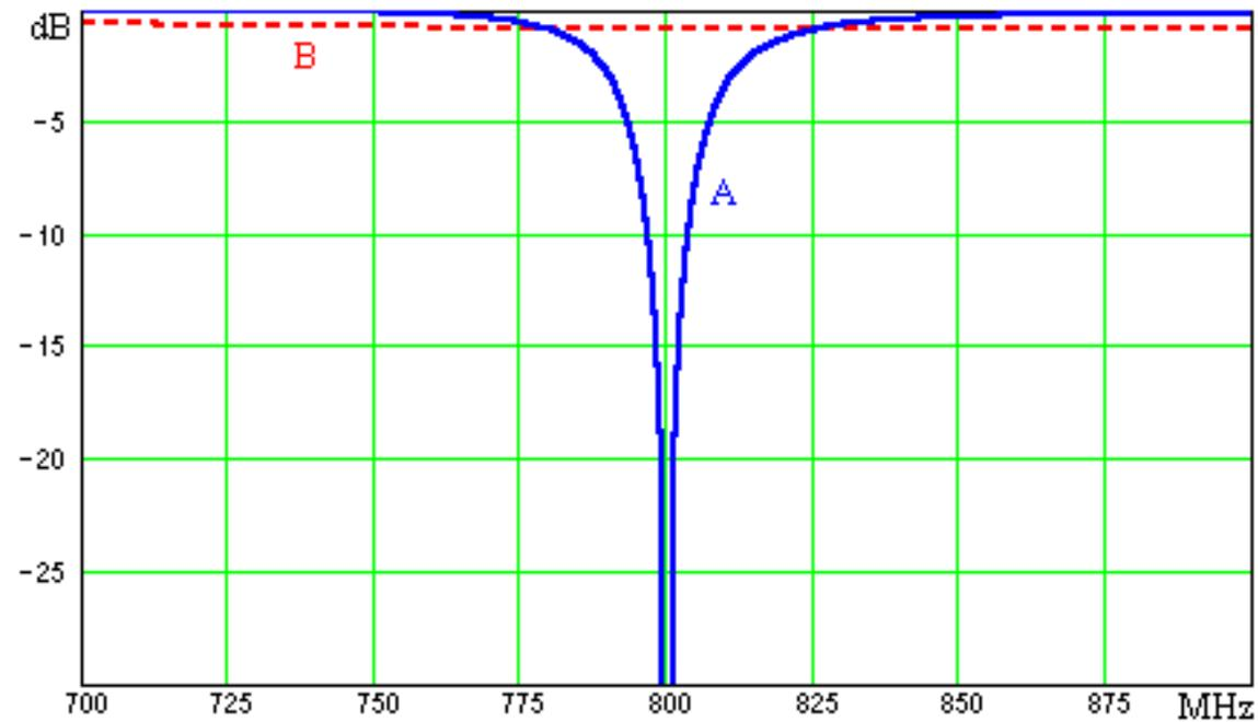
The return figure versus frequency, for the tuning at 800 MHz:
