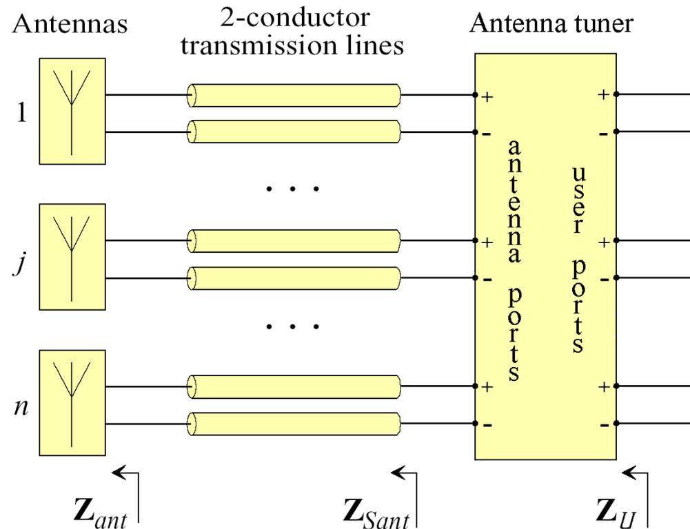
□ The MAPMUP antenna tuner allows an adjustment of  $Z_U$ , using a selection of the reactance values of its  $p$  adjustable impedance devices. Thus, it is possible to compensate a variation in  $Z_{Sant}$ .
