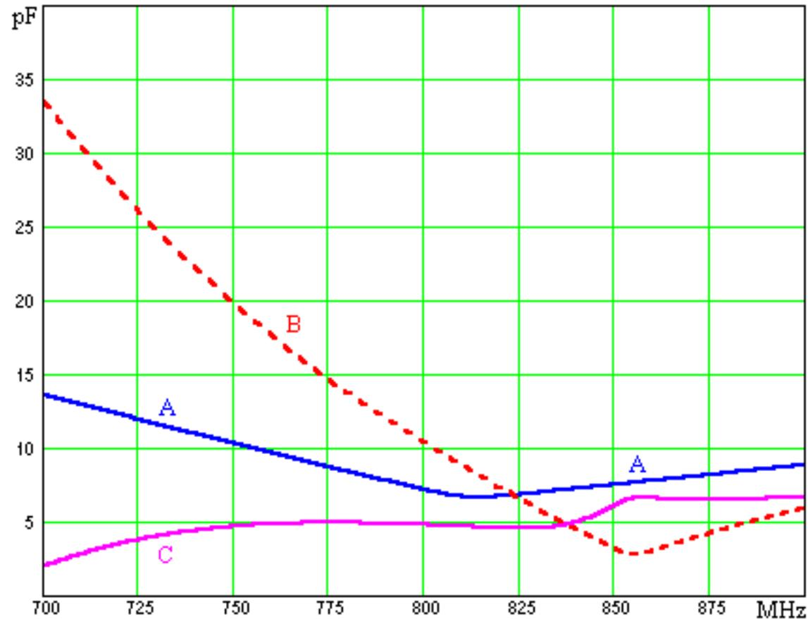
Capacitances of the adjustable impedance devices which realize  $C_U$ , versus the tuning frequency:
