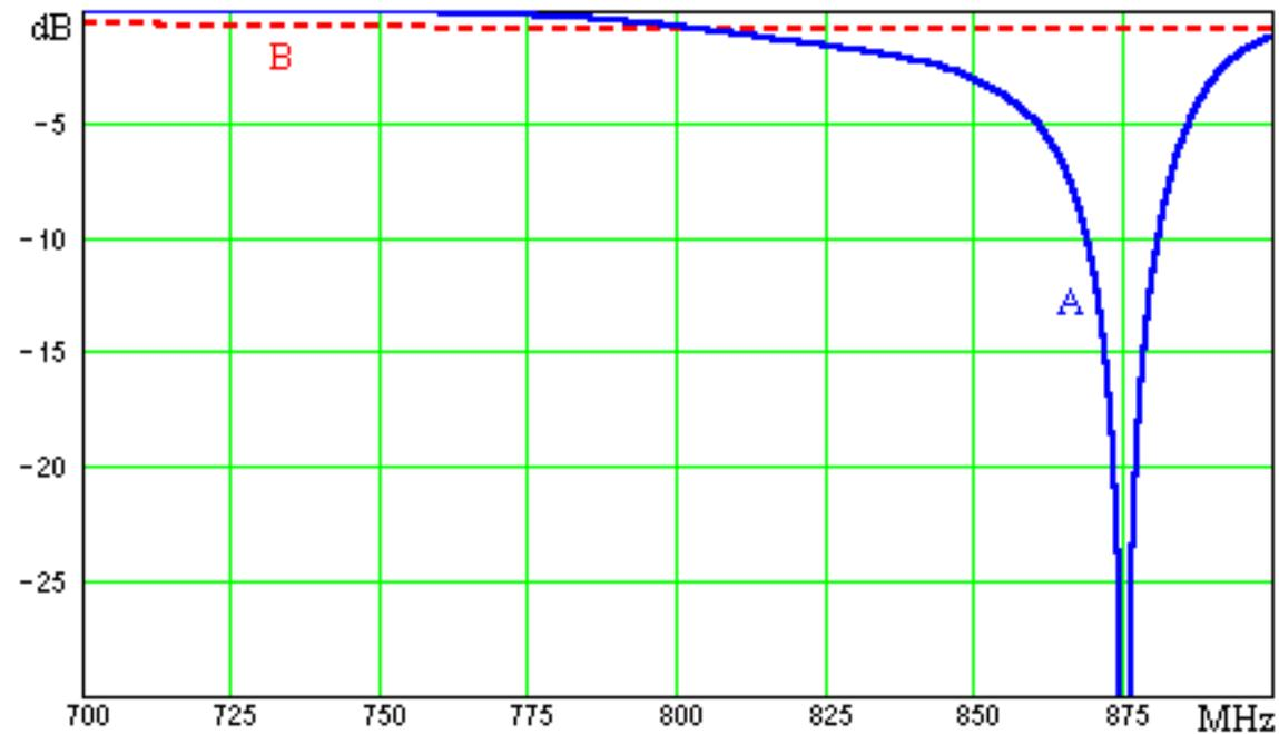
The return figure versus frequency, for a tuning at 875 MHz:
