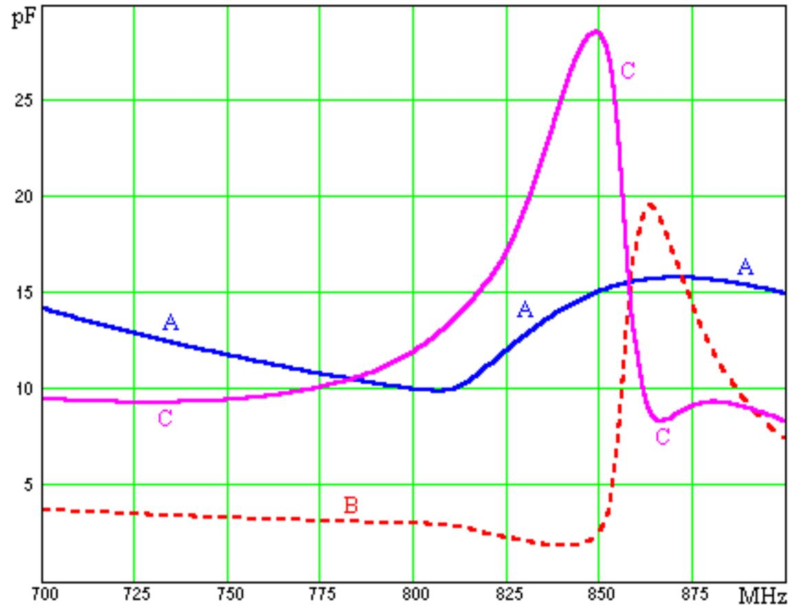
Capacitances of the adjustable impedance devices which realize  $C_A$ , versus the tuning frequency:
