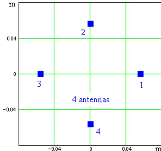
□ A circular antenna array made up of  $n = 4$  parallel dipole antennas is intended to operate in the frequency band 700 MHz to 900 MHz.
