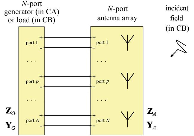
**FIGURE 4.** The two configurations, CA and CB, considered in Section VII.A for a multiport antenna array (MAA).
