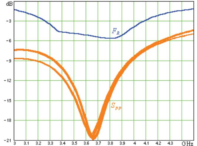
FIGURE 5. The return figure  $F_R$  and, for  $p \in \{1, \dots, 8\}$ , the absolute value of the entry  $S_{pp}$  of  $\mathbf{S}$ , computed for the 8-port MAA considered in Section VII.
