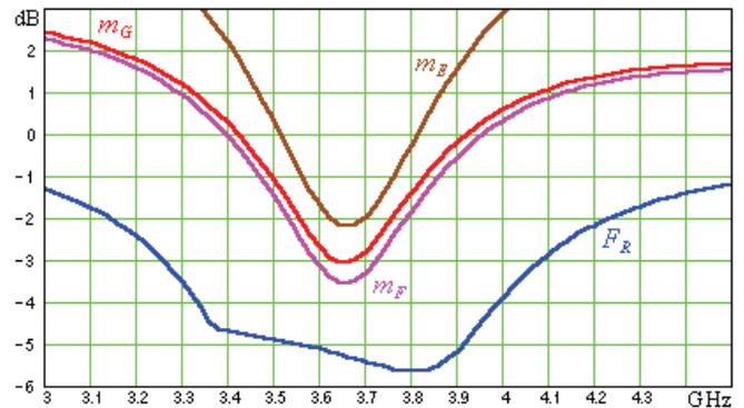
FIGURE 6. The return figure  $F_R$  and the upper bounds  $m_E$ ,  $m_G$  and  $m_F$ , computed for the 8-port MAA considered in Section VII.
